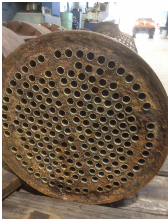
The cast iron face of the condenser unit was heavily corroded after 20 years of service
