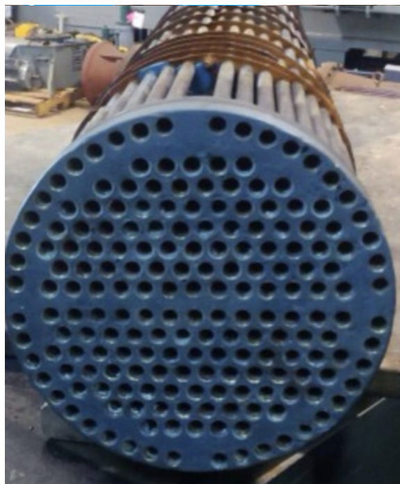
Ceramic Supergrade rebuilt the face, creating an ultra-smooth surface over the deformed cast iron with high resistance against future corrosion
