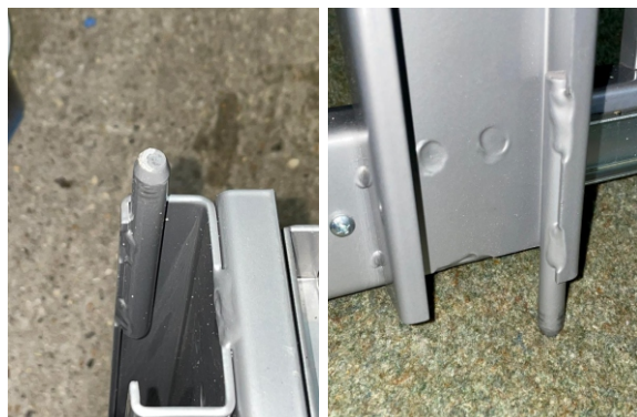
How the pin would have looked when it was welded to the unit before snapping off
