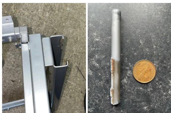
The part of the unit from where the 100mm pin had snapped off and the pin itself after it was detached from the unit
